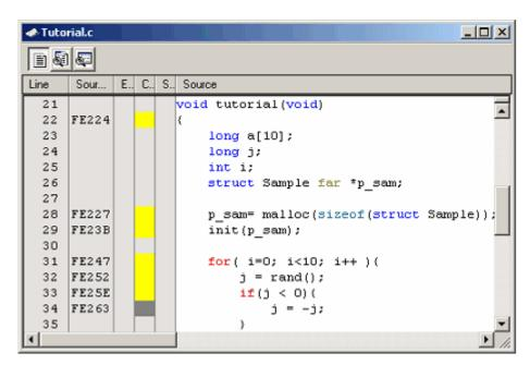
Figure 5.102 Example of code coverage results
